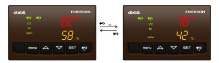
The variables (suction temperature, evaporation pressure, superheating value, opening value of the valve, etc.) that are to be viewed on the upper and lower displays are selected via the special parameter (Ec43 and Ec44).
